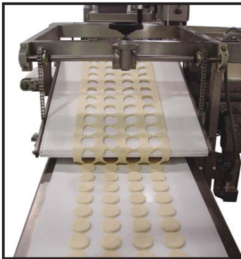
Removing Trim Dough Web From Cut Product
